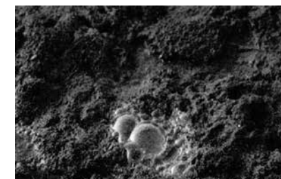
The second indication of the PLOCHER effect: formation of bubbles, as here in a size of 3 to 5 cm.
