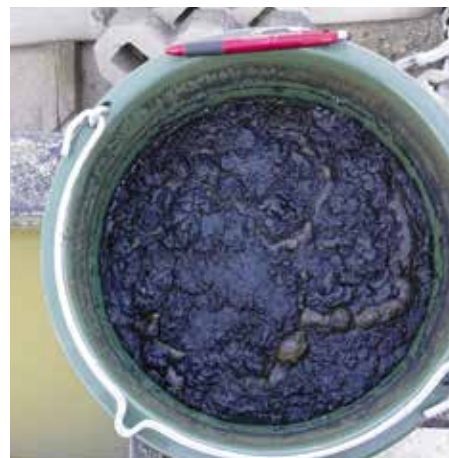
Digestate slurry treated with plocher digestate activator me after three weeks
