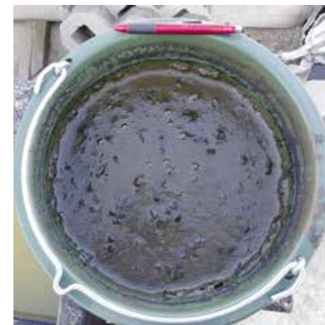
After short stirring: The sample is homogeneous with increased formation of fine bubbles, odour-neutral and of "creamy" consistency - aerobic active biology.
