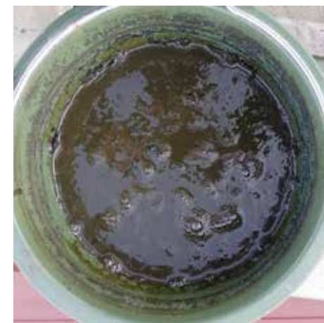
After a short stir The sample had a very unpleasant odour and the non-decomposed structures were still clearly visible. In terms of colour, this digestate slurry was inhomogeneous, blotchy and rather light-coloured.
